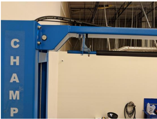
Overhead Safety Switch
