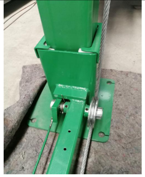
Conection way of lock release bar for manual lock release type
