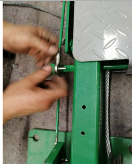
Conection way of lock release bar for manual lock release type
