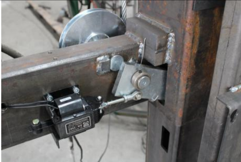
ELECTROMAGNETIC UNLOCK for electric lock release type
