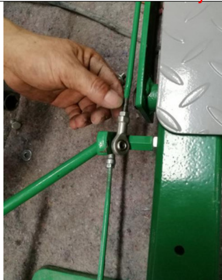
Conection way of lock release bar for manual lock release type
