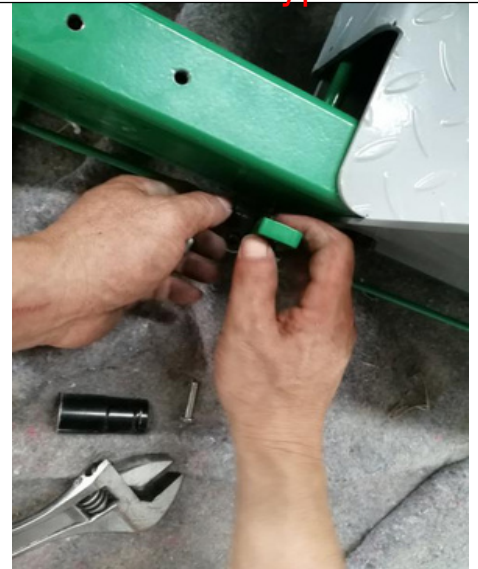
Conection way of lock release bar for manual lock release type
