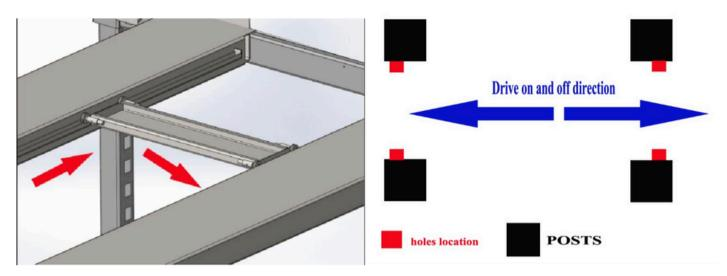
Recommendation:Our lifts are designed and manufactured in perfect performance,but wax the outside of the posts with paste wax or spray wax can reduce friction and keep smooth operation. Do not recommend to use grease,which will make it dirty.
