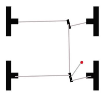
Note:This lift has 2100mm lifting height, if it is too high for you to touch the release handle when it stopped on the highest level, do not worry, there is a special design for the handle.You will find a small hole in the rod.You can please put a steel cable or rope through the hole and then you can easily touch it and release the lock.
